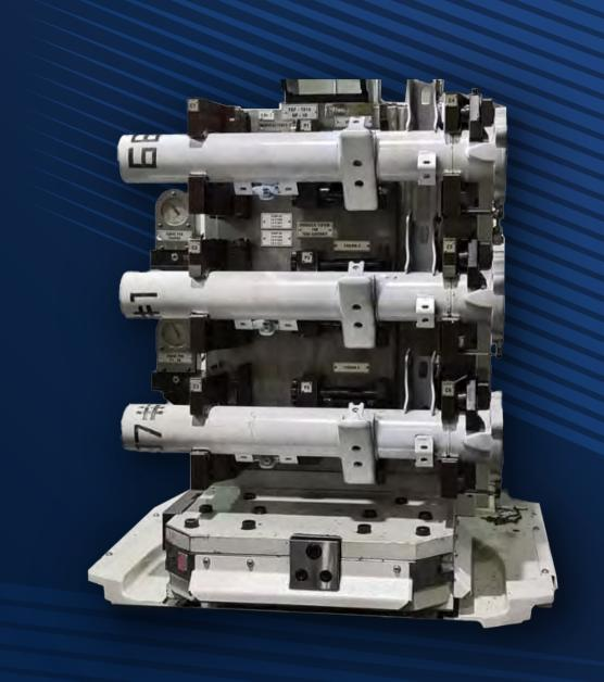
Multiple sets of high precision hydraulic fixtures supplied to a leading Tier - 1 automotive company in Thailand. The Company produces a broad range of products for passenger cars, pick-up trucks and agricultural machinery.
